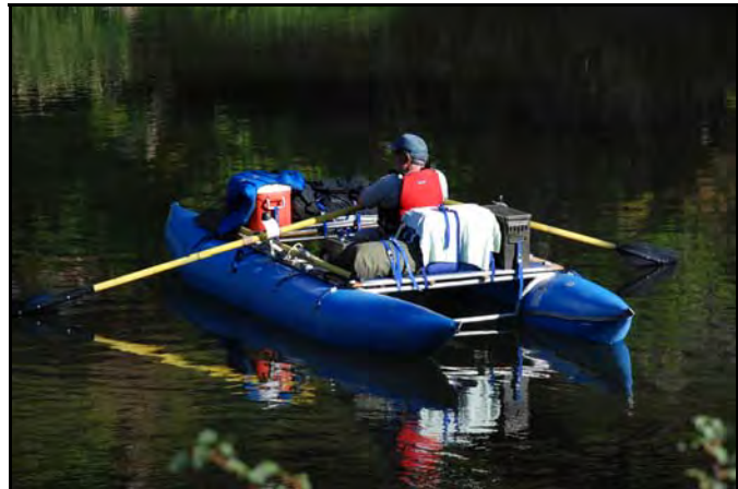
Figure 2.4: Cataraft – With their two tubes and frame in between, catarafTs are similar to catamarans. Middle Fork of the Salmon. Source: Author – [file:\DSC_0007.jpg]
