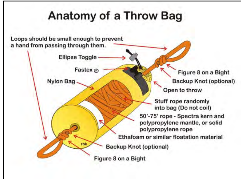
Figure 6.3: Anatomy of a Throw Bag – Caption: Throw bags come in many sizes and shapes. The bag diagramed is a typical bag used by the author. Remember to choose a bag that you will carry with you. Source: Author – [file: \BAG-AnatomyThrowbag.cdr]
