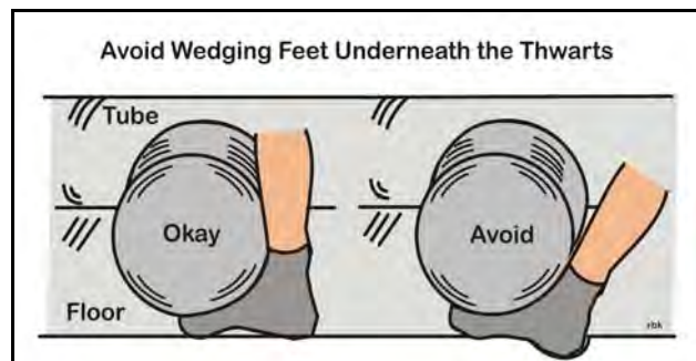
Figure 7.20: Throw Bag Drill – Excessive wedging of feet underneath the tubes can lead to paddler harm. Source: author – [file:\EQUIP_FootTubes.cdr]
